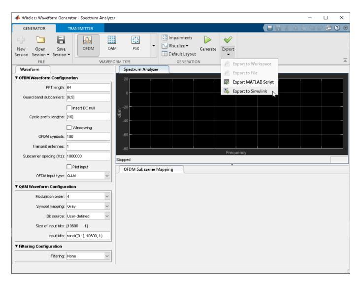
The **Export to Simulink** option creates a Simulink block, which outputs the selected waveform when you run the Simulink model. The block is exported to a new model if no open models exist.
