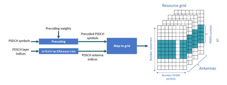
[~,pdschAntIndices] = nrExtractResources(pdschIndices,pdschGrid); pdschGrid(pdschAntIndices) = pdschSymbolsPrecoded;
