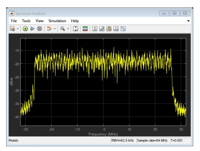
The Spectrum Analyzer block inherits the Waveform sample rate (Fs) parameter, which is 64 MHz.
