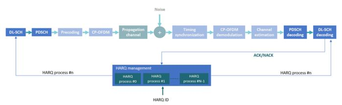
The examples also measures the block error rate (BLER) using an AWGN channel. This figure shows all of the link elements modeled in this example followed by the BLER calculation.
