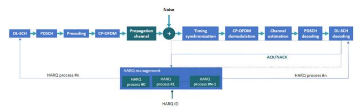
These examples show how to model the main elements of the downlink communication link. Modeling the main elements of the uplink communication link is similar.
