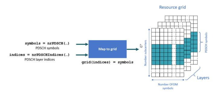
Because this example applies MIMO precoding to the PDSCH symbols before mapping them to the resource grids, the MIMO-precoded PDSCH symbols refer to antennas and not layers. To convert layer indices to antenna indices, use the nrExtractResources function. This figure shows the mapping process of MIMO-precoded symbols to as many resource grids as transmit antennas.
