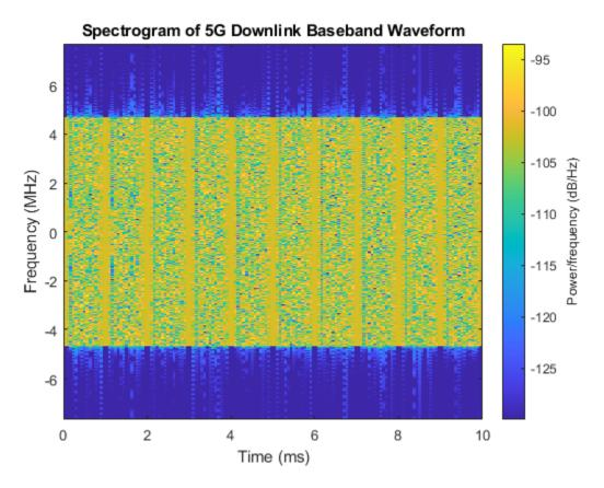
Change the PDSCH allocation to span PRBs 0 to 10. Generate the waveform and plot the spectrogram.
