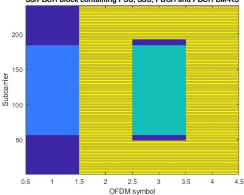
SS/PBCH block containing PSS, SSS, PBCH and PBCH DM-RS
