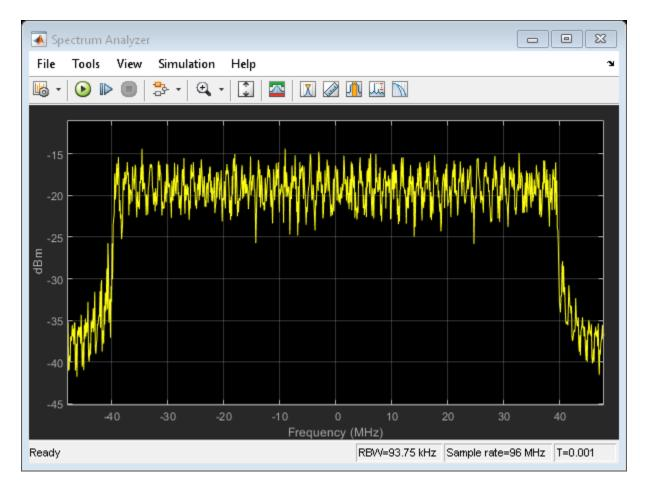
The Spectrum Analyzer block now shows a sample rate of 96 MHz, which is 1.5 times the previous sample rate, as expected.
